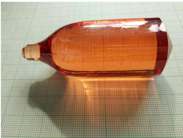
Fig. 1. Photo of the as-grown Sm:YAP crystal.
